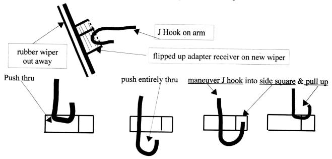
Push the "J" hook thru opening as shown. Keep pushing until thru enough to maneuver J hook into the little compartment. Then pull up until it stops. Rotate the blade parallel with the wiper arm. Push the adapter down until it locks into place.
