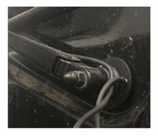
Tighten it to 12-14 nm of torque (approximately 8.85-10.32 ft-lbs).
