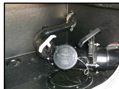
Figure 36 Thor Vegas/Axis Sewer Hose Connection and Black (black handle above) and Gray (white handle above) Dump Valves
