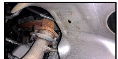
Figure 12 Transmission Cable Melted Through
