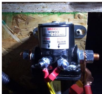
Figure 19 Electrical Coach Battery Disconnect Relay
