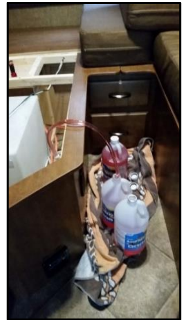
Figure 8 RV Antifreeze Configuration and Connection
