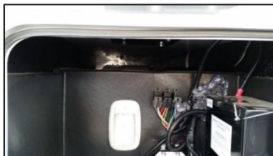
Figure 21 Battery Control Center Located under Driver's Seat in Storage Compartment (selected Thor applications)
