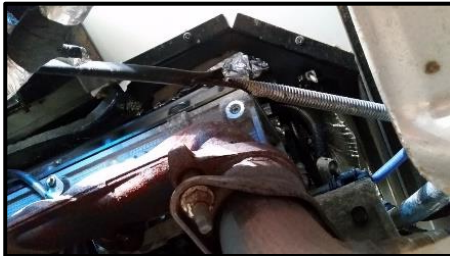
Figure 13 Transmission Cable against Exhaust Manifold
