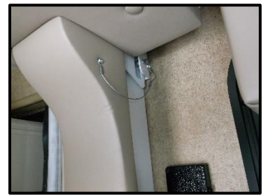
Figure 33 Front Bunk Safety Pin (Located on Driver's and Passenger's side)
