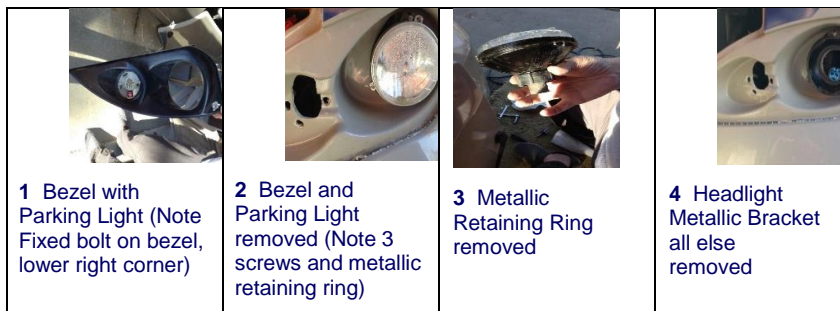
Figure 77 Headlight Removal
