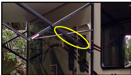
Figure 42 Awning Side Arm Latches to Lower End of Awning to Drain Water
