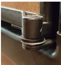
Figure 80 Door Reinstalled with Hinge Reinforced
