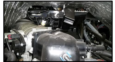
Figure 56 FatMat Insulation Added
