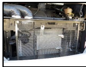
Figure 70 Radiator and Oil Cooler Protection Mod
