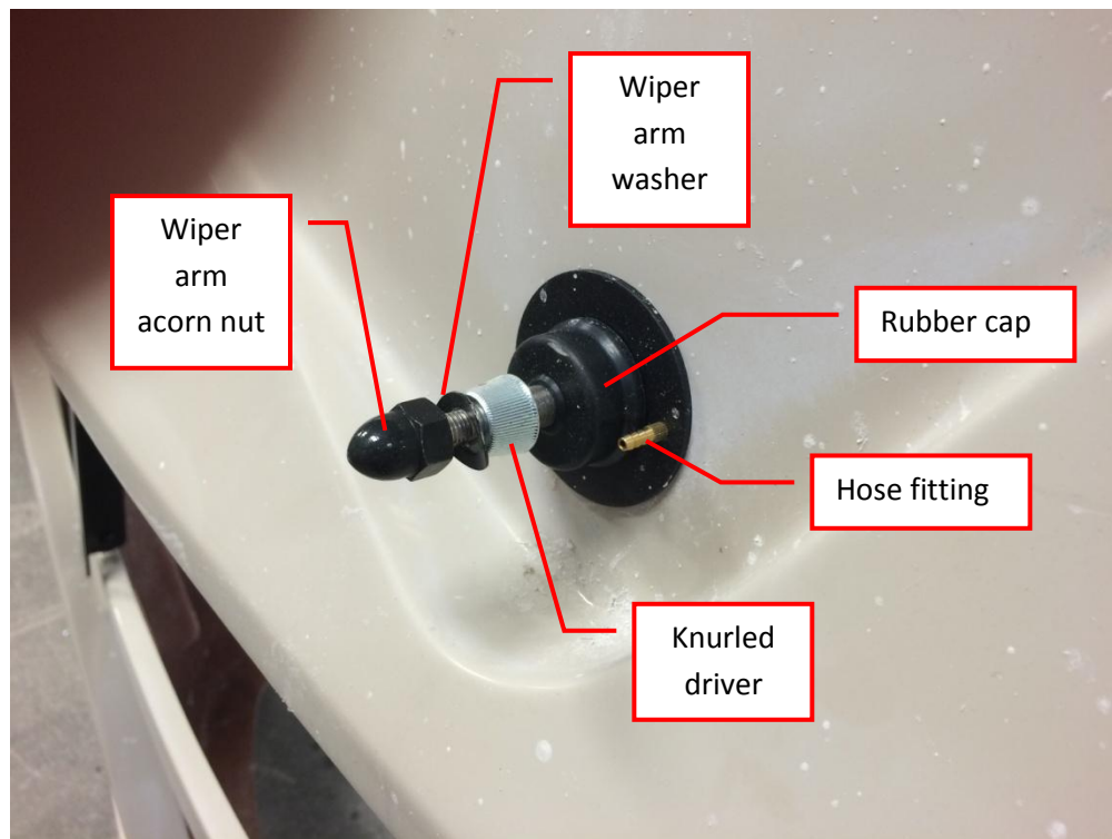
Fig. 1 Pivot shown with arm removed and washer hose disconnected
