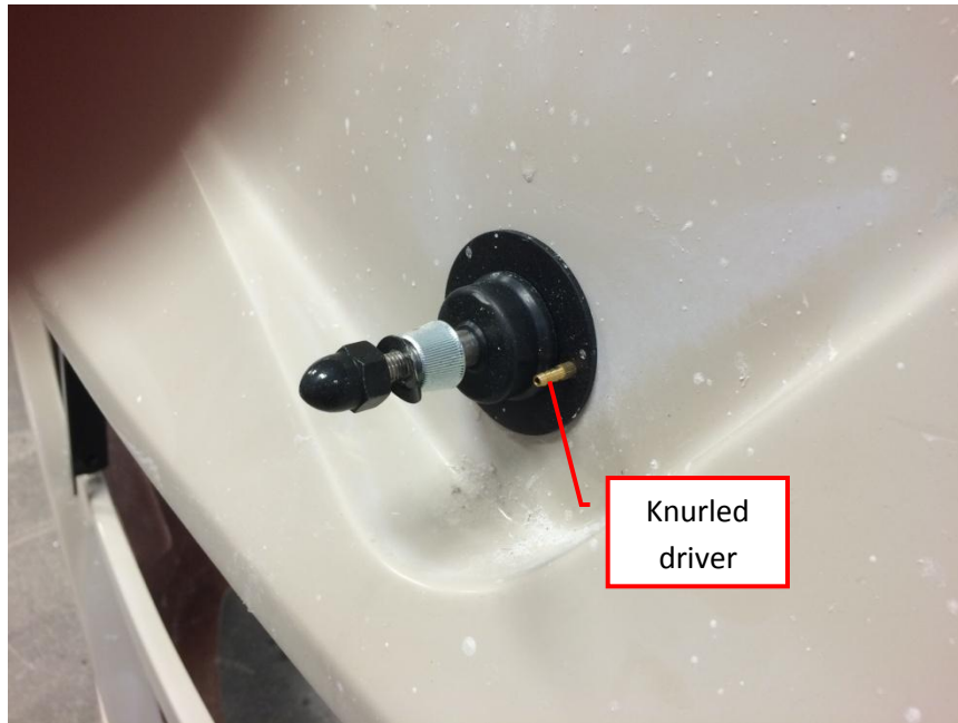
Fig. 2 Pivot shaft with arm removed
