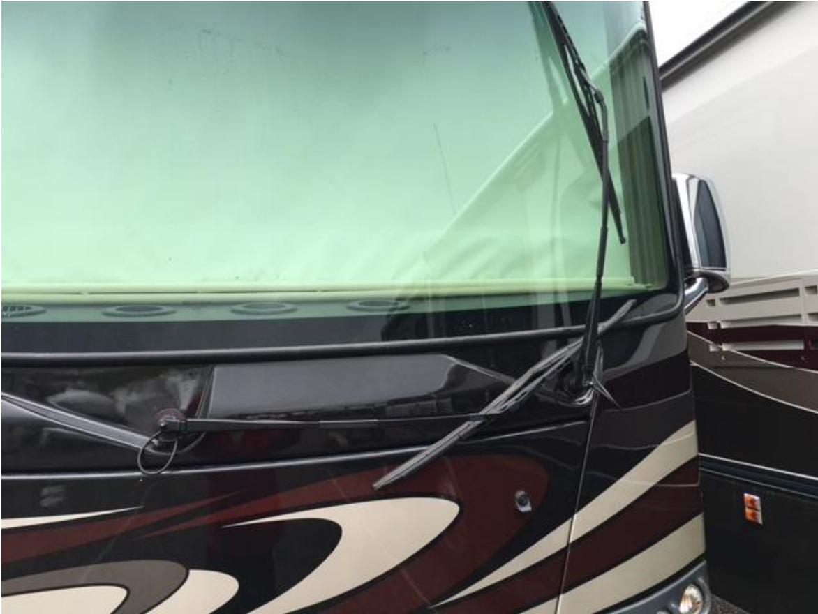
**Linkage toggle causing passenger side arm to over-travel and jam
