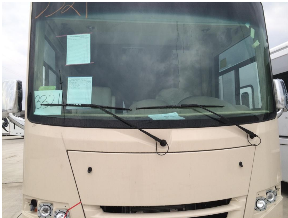
Fig. 4 Correct typical wiper arm park position
