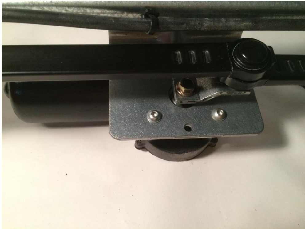
Fig. 3 Correct park position of the wiper linkage
