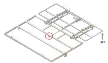
With the bed in the full upright position a hole in the frame will align with a hole in the frame support roller. Insert the clevis pin used for the actuator connection through the roller and frame tube to lock the frame in the up position. Be sure to use the cotter pin with the clevis pin to keep the pin in place.
