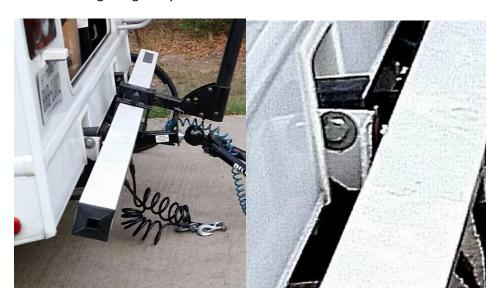
This was not the fault of the adapter. It is the fault of the ultra-thin bumper on my RV, the extremely rough roads in Oklahoma and the fact I loaded three heavy bikes on this vibrating assembly and did nothing to stabilize it.
