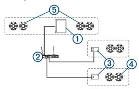
In the image above, one RV-IN1501 stereo ① connects to a wireless router ② and to two Apollo SRX400 zone stereos ③. The two FUSION PartyBus stereo zone stereos can stream sources from the FUSION PartyBus stereo.
