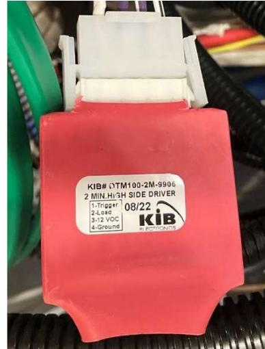
3. Replace the timer if needed, timer connector is directional and will only connect one way.
