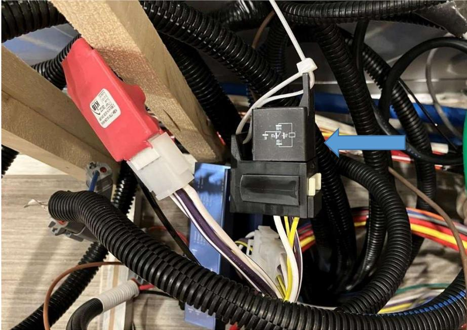
2. While holding the relay, apply a load to the microwave circuit.
