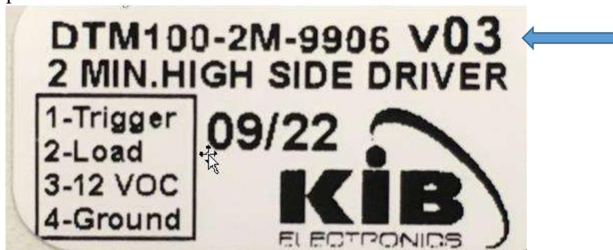
2. The date code on timer sticker can also be used to indicate if the module needs to be replaced.
